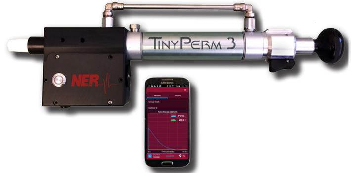
The measurement data, along with GPS-derived latitude and longitude coordinates, serial number of the TinyPerm permeameter, date, barometric pressure, ambient temperature and humidity, and sample images, are captured in data files that are easily exported from the Android device to desktop computers for additional analyses.
